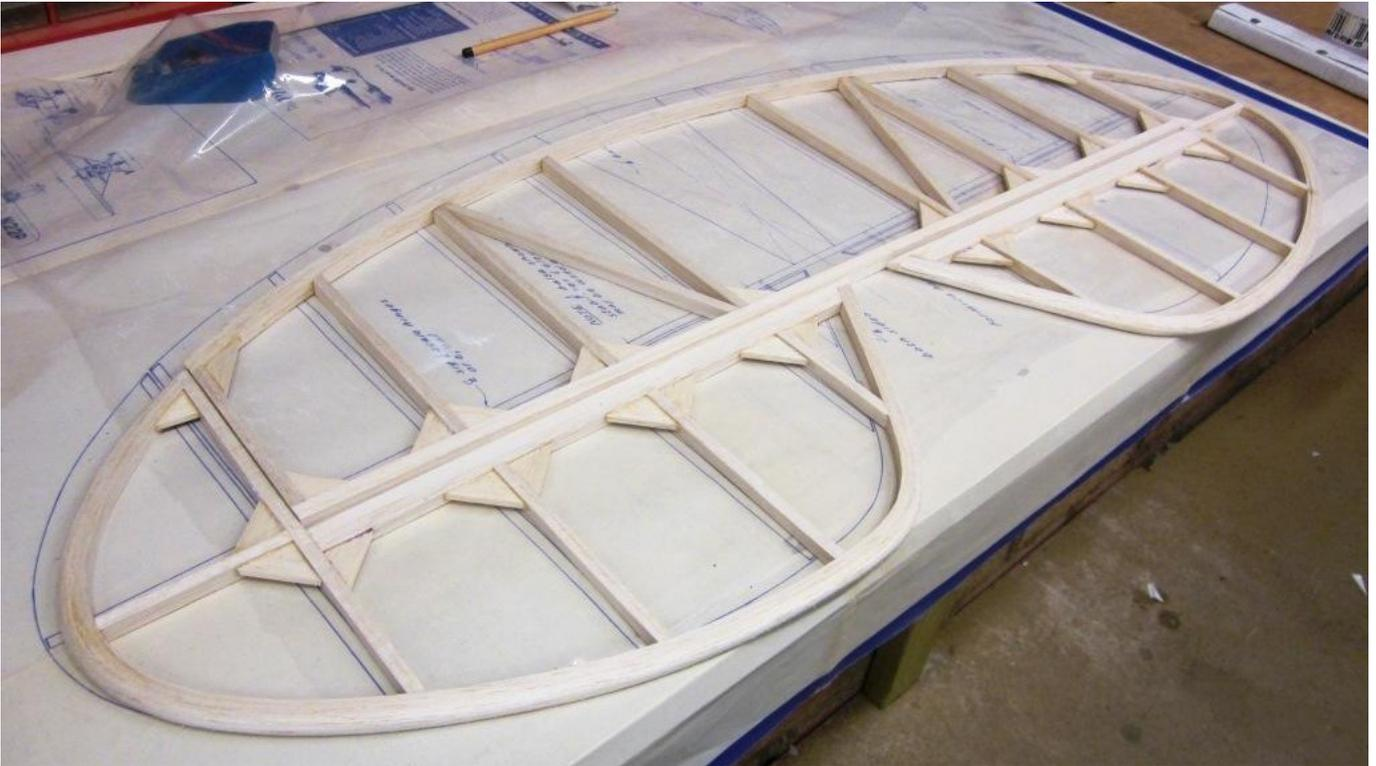
The stab and elevators are more or less finished now but I still have to work out a way to mount the stab as per the full size which pivots on the elevator hinge line with the incidence being trimmed for hands off flight at the leading edge, from memory there was about a 25mm gap between the inside end of each stab and the side of the fuselage.
