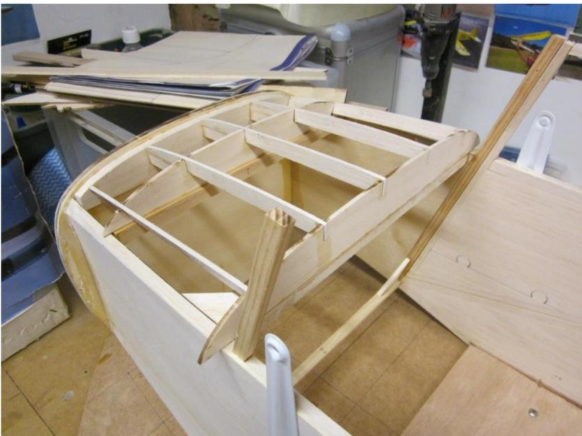
The plans don't show any way of mounting the stab and fin so I'll have to make up something there as well and it too will need accuracy with having the stab level and with the correct angle of incidence.
