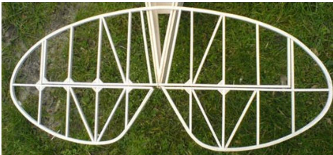
The solid parts that Brad has supplied wont go to waste as I can use them for formers to bend laminating balsa strips around.
