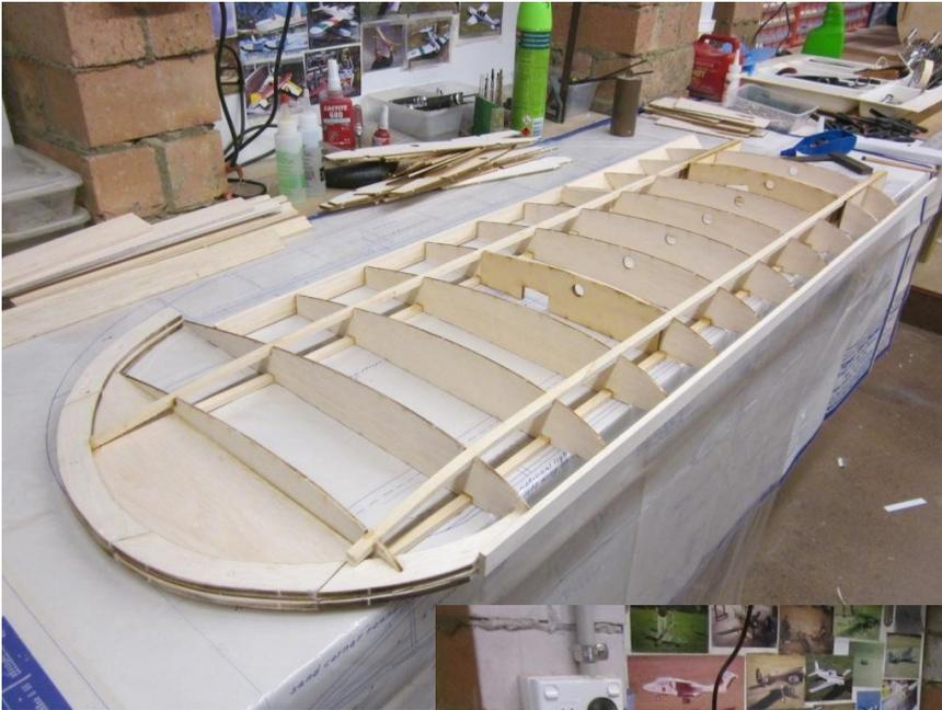
It's a pretty simple wing and easy to put together with laser cut parts. The starboard wing was made first and then the port wing was made.
