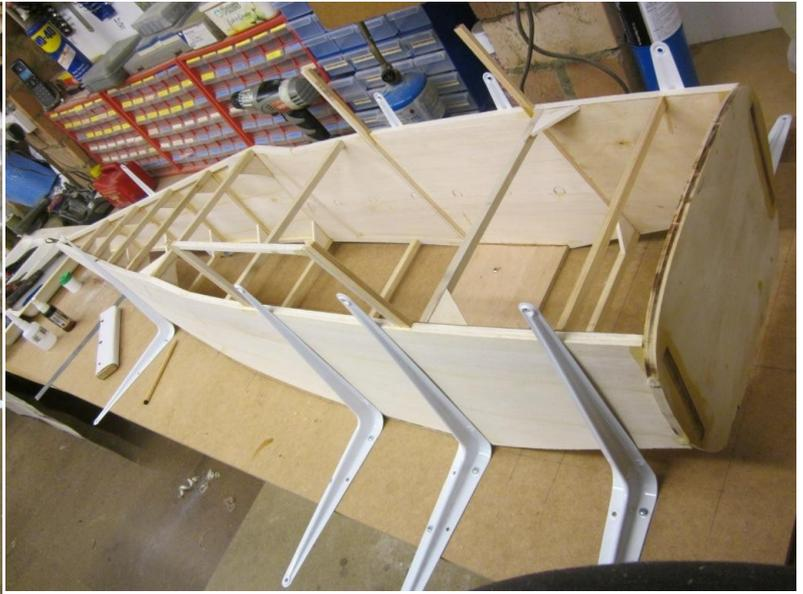
Cross members and frames are fitted and the fuselage is now rigid and ready for the wing mount, longerons, frames and planking. I'll leave the fuse in the jig until I have finished the wing mount as it will be critical to get the mount level with the right angle of incidence.
