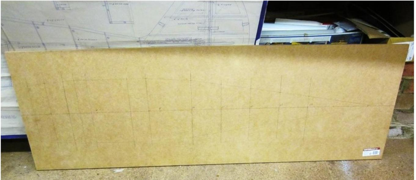
A centreline was drawn down the MDF sheet and the outer profile of the fuselage was plotted from the plan at each frame point. The position of the undercarriage plate was transferred to the jig and the fuselage was screwed to that position through the U/C plate.
