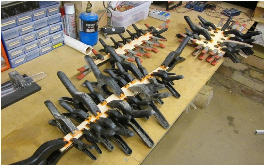
These bits are the wing joiners, main U/C floor and firewall all glued with Tite-bond wood glue.
