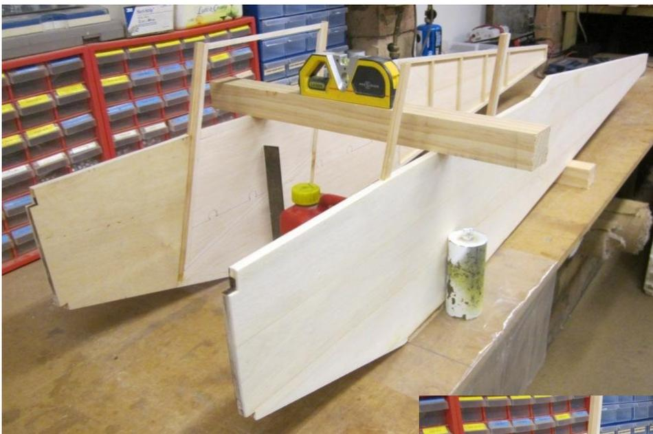
The two sides will form a box like structure that will have frames and stringers attached to the outside to form the fuselage shape.
