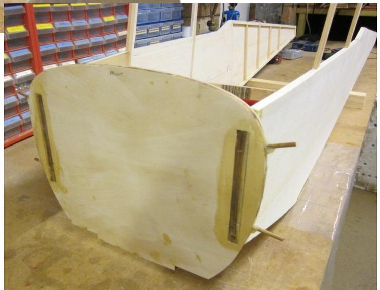
The next challenge is to fit the cross members and frames but after a preliminary play it was obvious that if I wanted a square and true fuselage I would have to make a jig the full length of the fuselage to ensure the sides were vertical and followed the overhead profile on the plans This was a bit of a hassle as the jig had to be made from a bit of MDF 1800 x 600 x 16mm and 12 x 300mm el cheapo right angled brackets.
