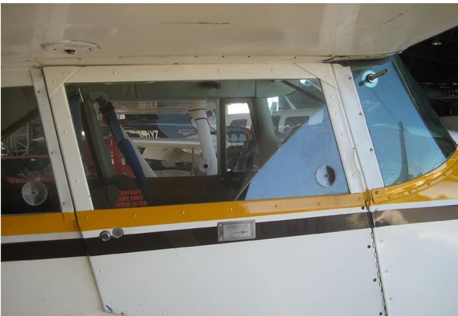
The pilots door is in front of the wing struts so has to have the diagonal bottom sill for clearance.
