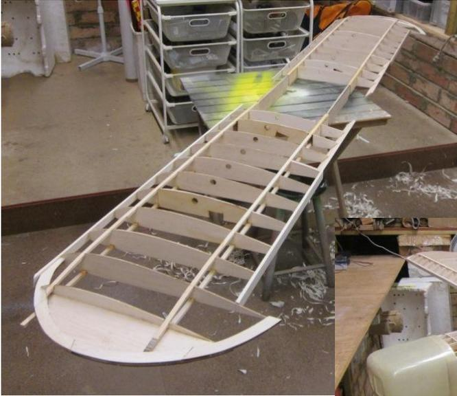
The wing joiner beams are two large pieces of 3/8" aircraft grade plywood that have to be fitted into the wing mount boxes made up in the root of the wings. Careful sanding and shaping enabled me to get the first look at how big this thing is.
