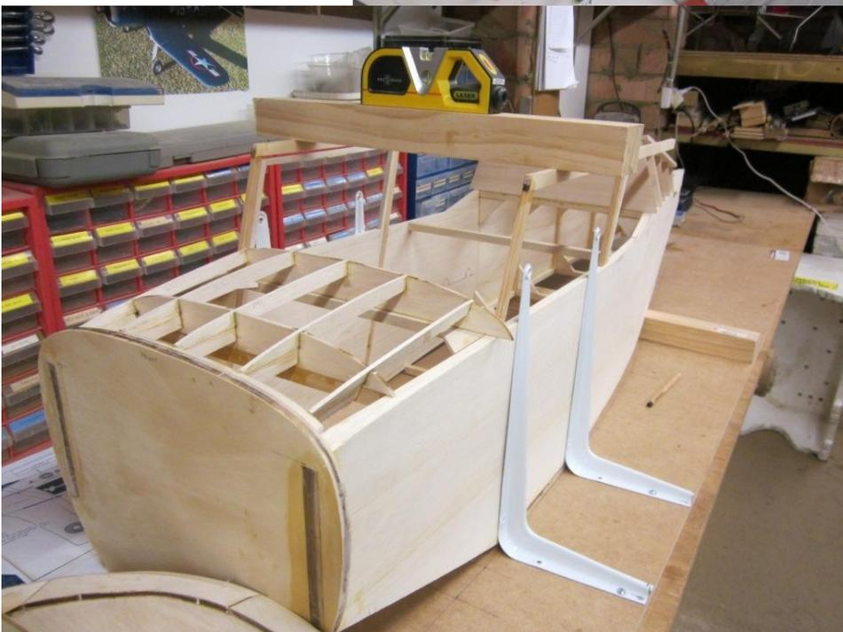
now up to making the wing mount on top of the fuselage.
