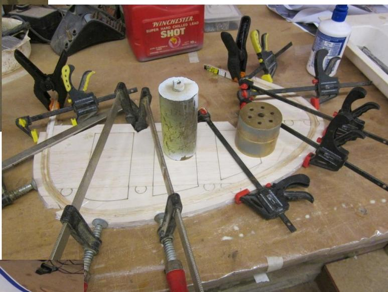
I used 8 laminations of 1/16" balsa glued with ordinary old Aquadhere and left overnight in the jig to cure.
