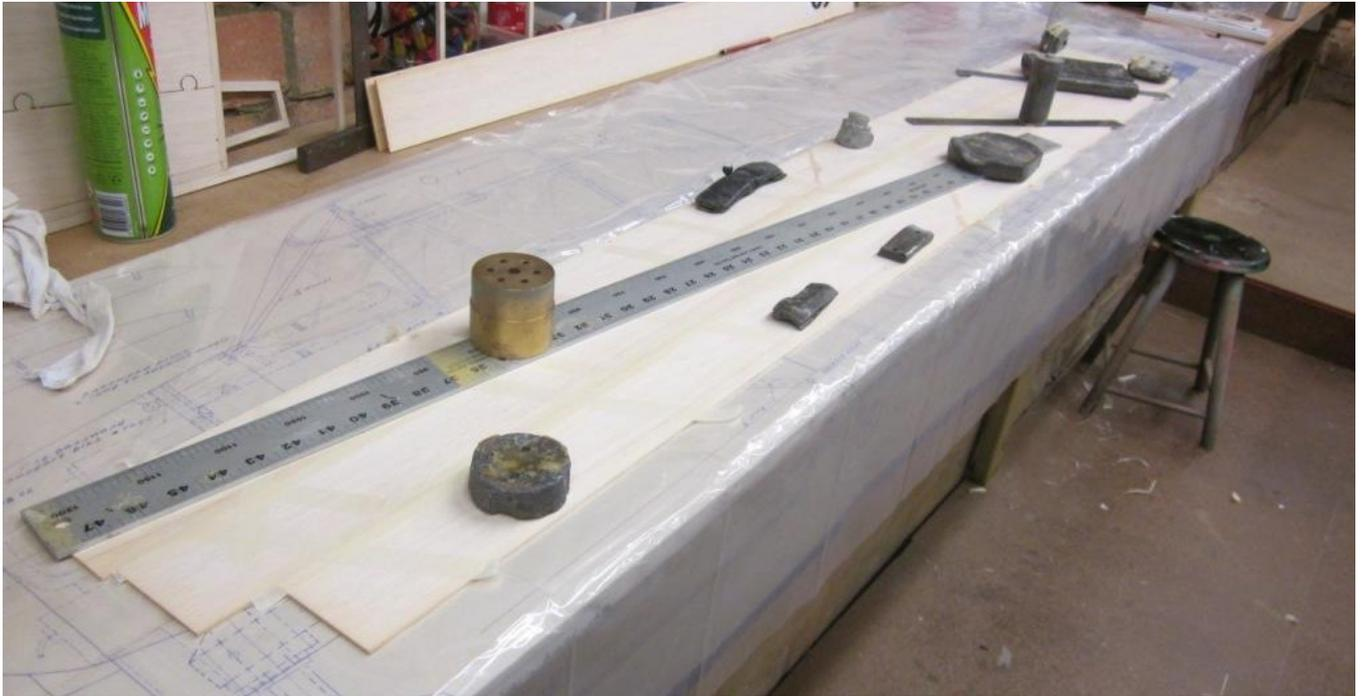
The picture above shows 6 sheets of 1/8" x 3" x 36" scarf and butt joined to create the large sheet required per side.
