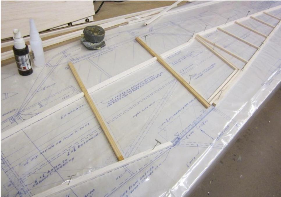
The fuselage construction is a little confusing. The start is a balsa stick frame with solid balsa fitted between the framework to just behind the cabin and then the sides are completely sheeted on the outside with 1/8" balsa sheet.
