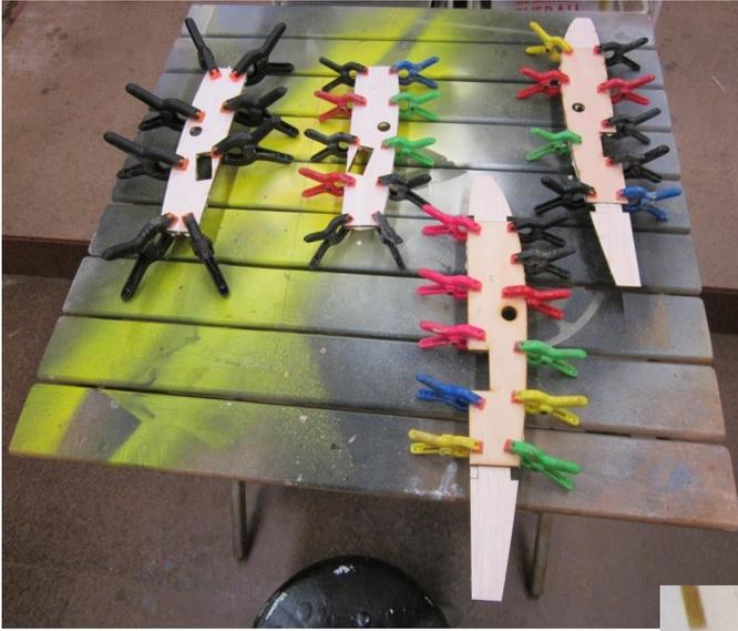
First step as usual with laser cut kits is to laminate all the parts that require extra thickness or strength. I use PVA and plenty of clamps and job done. One thing I have learnt along the way is it is far easier to wipe surplus glue off when wet using a wet rag than it is to have to sand it off when dry.
