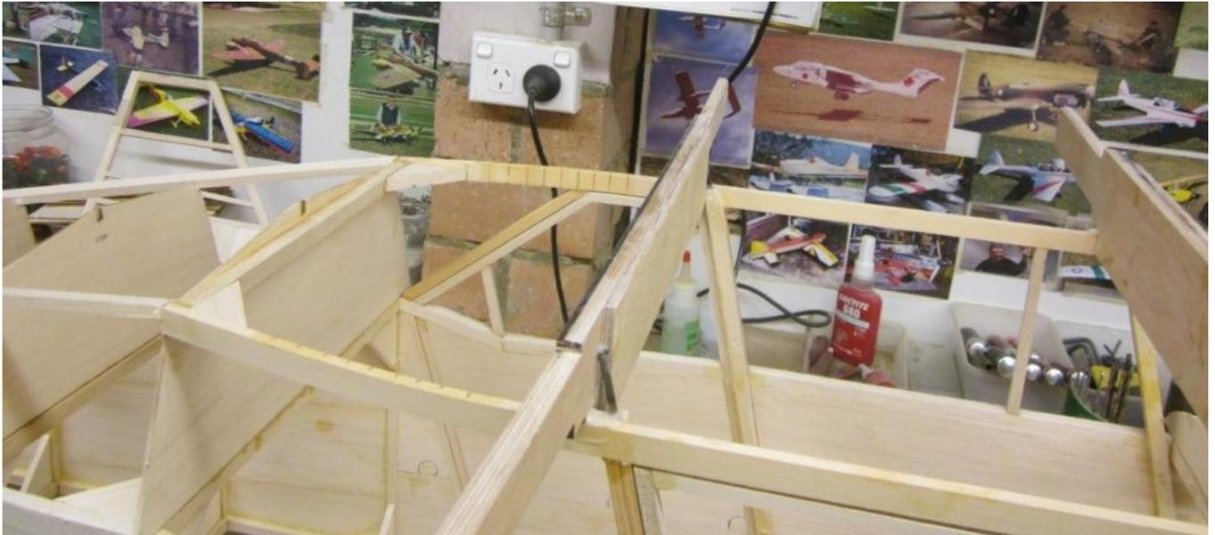
The back of the lengthwise cabin beams had to have a number of saw cuts to half thickness to be able to bend to join up with the first of the rear deck frames. Decent size 3/8" gussets with CA worked well here. To finish up, all the saw cuts were filled with thin CA.
