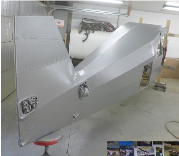
This picture of a full size Tri Pacer being restored well demonstrates the fabric finish over the longitudinal parts of the frame and fin.
