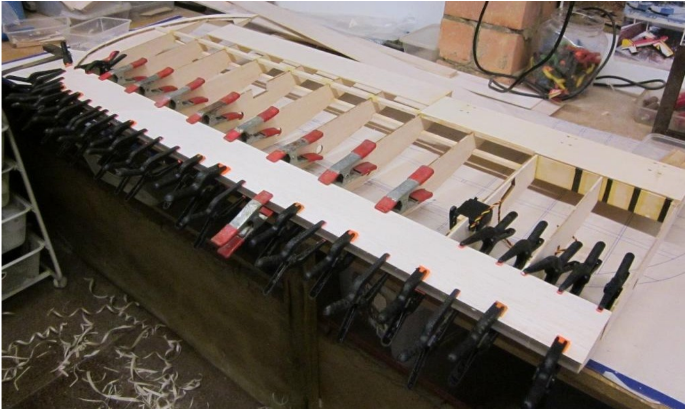
L.E. Sheeting on underside in place. These cheap Chinese plastic clamps make life easy.
