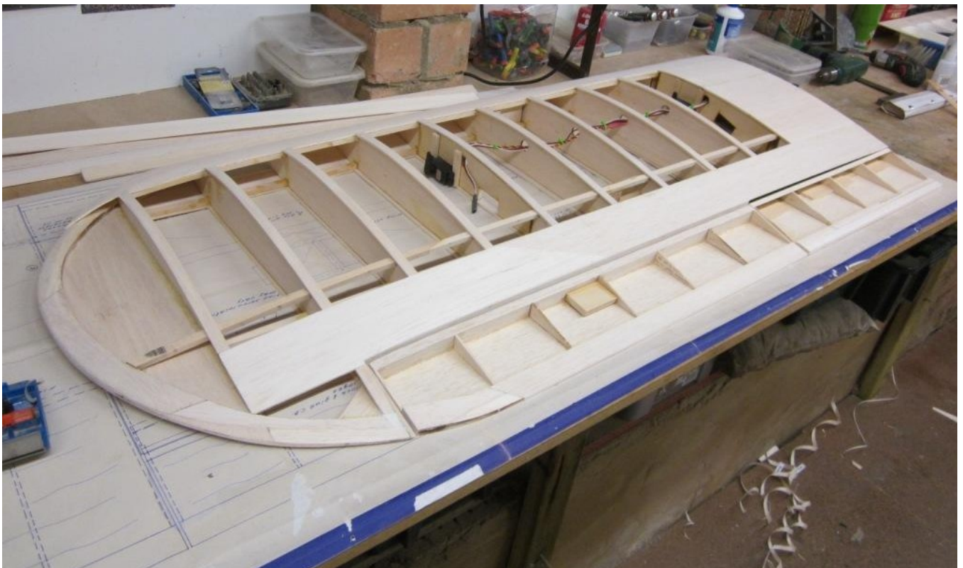
The wings are well on the way now, next job is LE capping and shaping, trial fit ailerons and flaps, fit nav and landing lights. I have cut out a section of the leading edge for landing lights and will need to cut a path for nav light cables
