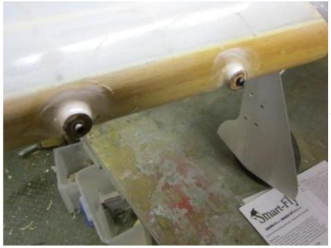
I built up the void with my usual mixture of bog and removed the cap screws when all was set.
