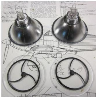
The landing lights are made from the lenses and reflectors from two \$2 plastic torches. I've discarded the incandescent bulbs and glued white LED's into the back of the reflectors. The black replicated bulb carriers that came with the Mick Reeves instrument panel kit were glued to the clear lens covers. The covers were then glued to the reflectors and trimmed to size, flexi lead soldered to LED, voila! All done.
