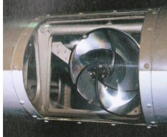
This is done by stapling sheets of 0.6mm clear PET sheet to two sticks, heating the PET with a hot air gun until floppy and then pushing it back over the leading edge and waiting for it to cool.
