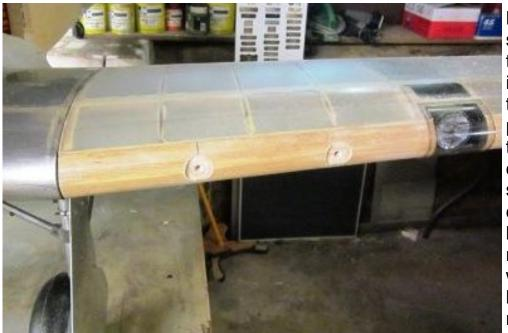
Because the canons stick out so far from the LE of the wing it is imperative that they are mounted parallel to the axis of the aircraft. This caused a bit of head scratching until I came up with counter boring the LE to give me a flat surface to work off and then hammering 8-32 T-nuts into the centre of
