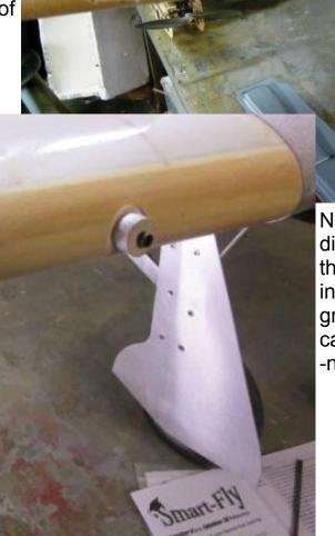
Next I epoxied a disc of dowel over the T-nut and held it in place with a well greased short 8-32 cap screw into the T-nut.
