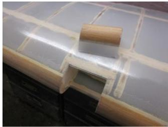
The wing leading edge is cut out to the internal framework and a light mounting plate glued vertically. The recess is painted with flat black and a silver painted plastic tube is glued above and below the reflector to look like the full size framework. The clear cover is glued over the lot
