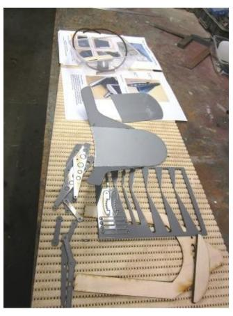
Another one of Micks kits, again made from laser cut plastic sheet. The chair is bent to shape and the glued and screwed together with a bit of softwood to reinforce the base. Very easy way to make a good looking scale chair. A coat or two of Cockpit Green finishes the job.
