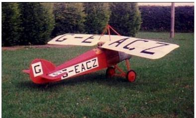
To quote Wikpedia ....." the Sopwith Monoplane No. 1, also known as the Sopwith Scooter. It used a normal Camel fuselage, with the wing mounted just above the fuselage, with a very small gap. The wing was braced using RAF-wires (i.e. streamlined bracing wires) to a pyramid shaped cabane above the wing. It was powered by a single 130 hp (97 kW) Clerget 9B rotary
