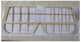
So now we have a fuselage and it's time to build the tailplane using the previously made tips, some 1/8 ribs, a  $\frac{1}{4}$  sq hardwood spar (from Bunnings) and balsa strip L&T edges. Notice the gap at the front - it has to fit around the end of the fuselage decking and until that is
