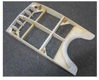
the landing wires will be attached. When they are all laid out they make up the 79" span (it was supposed to be 80" but I guess I got the enlargement of the free plan wrong!)
