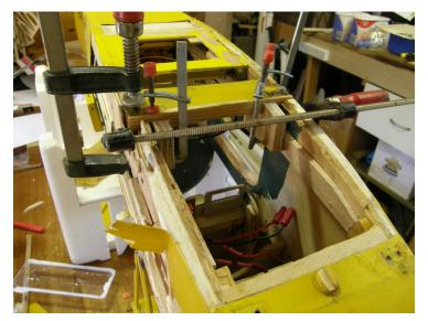
I started by grafting the new upper longerons into the rear portion of the fuse using epoxy, clamps and screws.
