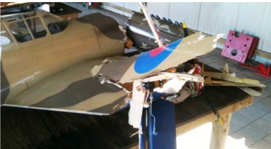
Half the planking on the port side had been ripped off with the cowl so new 6mm planking was grafted into the old and a new ply former laminated up and glued to the edge of the new firewall.
