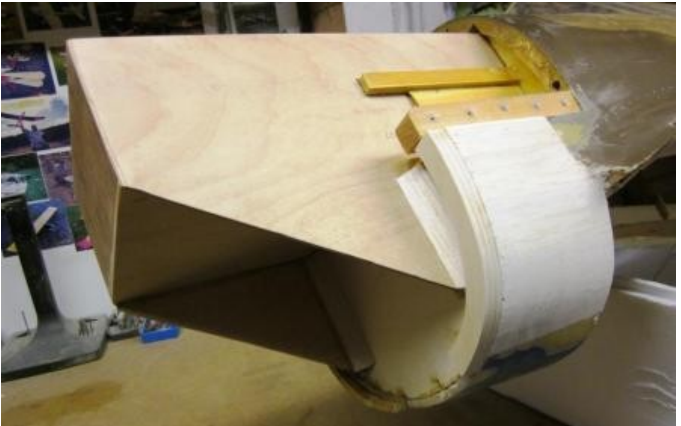
Half the planking on the port side had been ripped off with the cowl so new 6mm planking was grafted into the old and a new ply former laminated up and glued to the edge of the new firewall.
