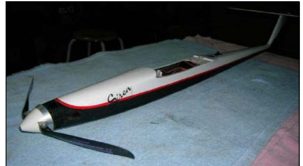
The length of the cowl of the Siren fuselage made for difficulties in installing the motor ( see article)
