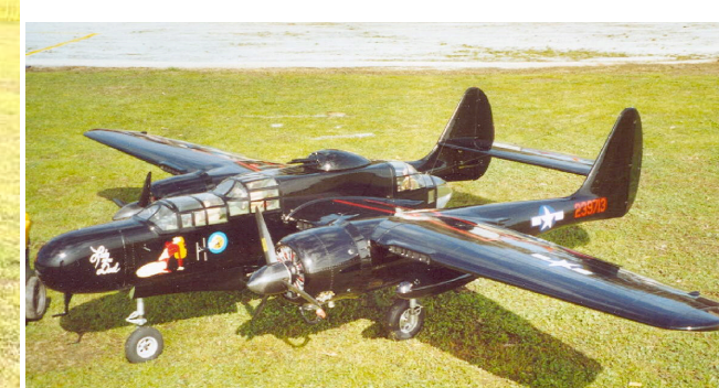
The CG turned out to be in about the right position but when I tried a test glide I seemed nose heavy so I moved the battery back a bit on it's velcro strip and it seemed better. Time to fire up the motor!
