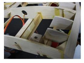
C/S in ply boxes - not very elegant but functional. The block of wood to the right with the hole in it is
