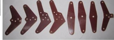
servos (one for rudder, one each for elevators) and the rudder. Here they are cut from PC board ready for installation (the holes in the centre are to make sure the epoxy keys in well).
