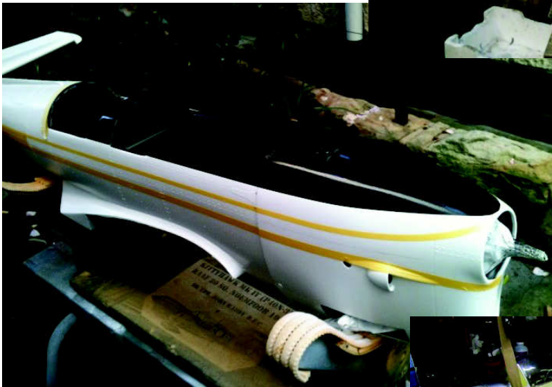
The black anti glare panel is done and next is the bright red flash down the fuselage sides, across the wing and fin.
