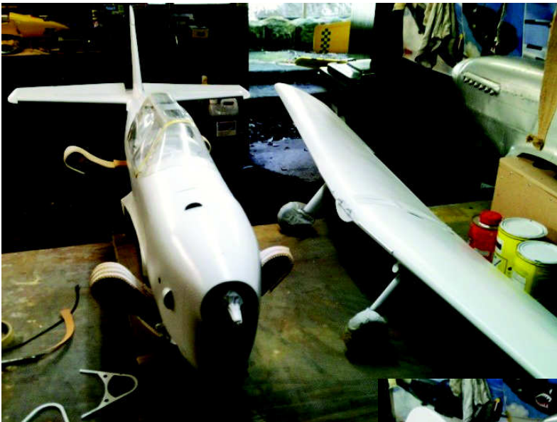
The white base coat is on and the canopy framing is work in progress.
